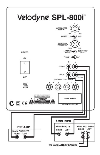
Figure 2. Installation Using Stereo Line-Level Inputs
